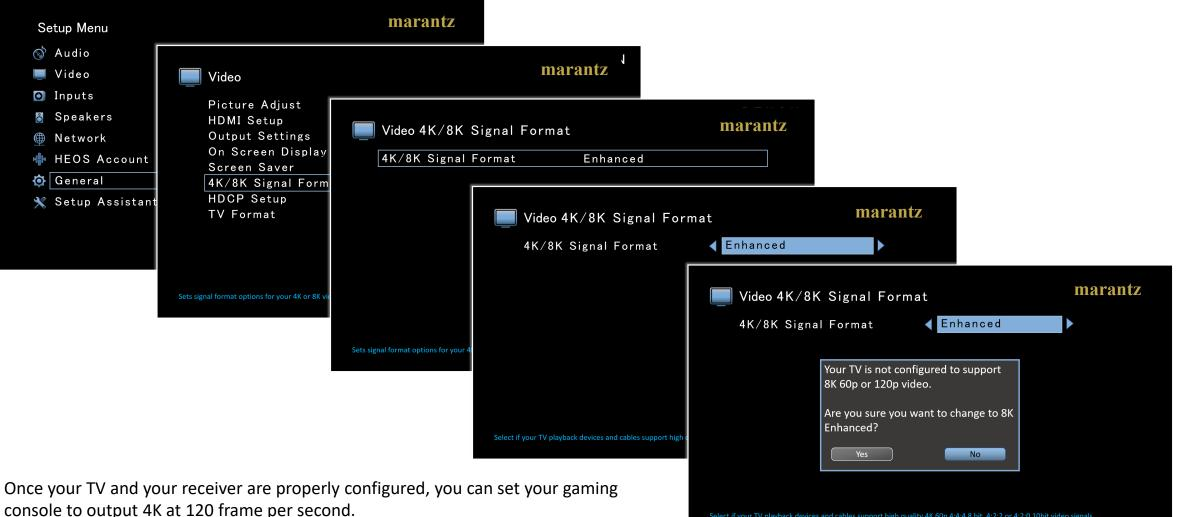
Select if your TV playback devices and cables support high quality 4K 60p 4:4:4 8 bit, 4:2:2 or 4:2:0 10bit video signals
